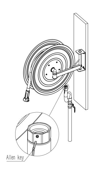
STEP 1 : take the tool and loosen the small locking screw.
