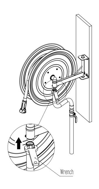
STEP 2 :connect the inlet hose with hose reel waterway and fix them tightly.
